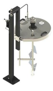
This elevator-agitator for 20-40 to 200 Liter drums features a double-effect jack for a fast lift of a stainless steel cover fitted for a quick material drum change. The cover is equipped with a motorized agitator fitted with blades for low viscosity materials and a full stainless steel rod. The elevator is coming on a large fixing plate which makes it very stable and easy to install in paint kitchens, existing installations or an essential component of new installations
